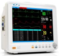
12.1" high resolution color TFT display ECG, SPo2, Respiration, NIBP & Temprature S-T segment analysis, pace-maker detection 3 level audio/visual alarming 6 hours battrey backup 7 days trends chart in storage
