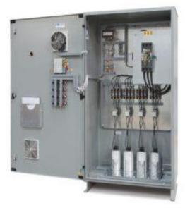
Power Factor Panels are constructed in steel-plate cabinets (vertical construction mounted type by smaller power ranges). The Panels are equipped with Automatic Power Factor Controller regulator, switching contactors, MCBs, Cylindrical capacitors Brands like EPCOS, ABB, SCHNEIDER ELECTRIC, L&T and fuses.
